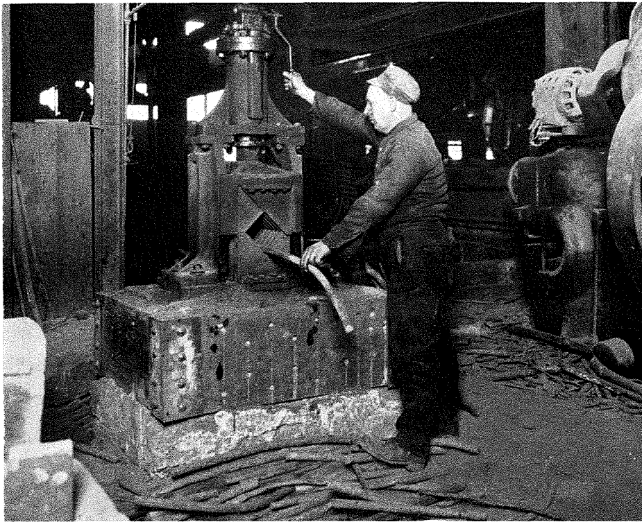
Crooks are quickly put on the straight and narrow at Continental Foundry and Machine Co., Wheeling, West Virginia. They haven't got a chance. It only takes a few seconds to put a crooked core rod in this Type "D" American Rod Straightener and Shear Machine, and turn the handle operating the compressed air. The dies make a four point landing, and the crooks are gone!
